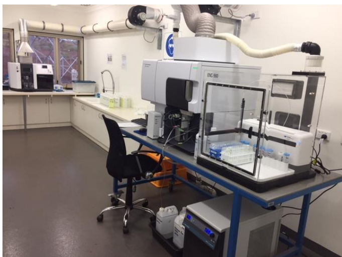
Photo 7. Inductively Coupled Plasma Optical Emission Spectrometer
