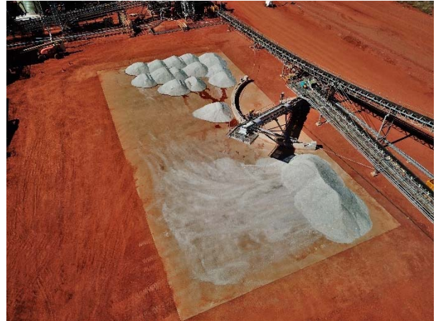
Photo 6 Lithium Concentrate Product Stockpile Pad
